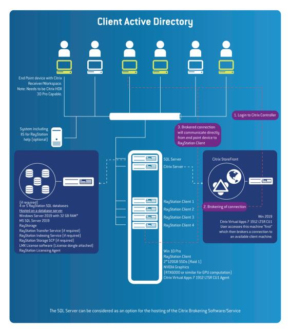
Figure 2. Central Ray Station with virtual desktop connection. \*Note that RAM DIMMs should be installed to provide optimal RAM usage, i.e, units of 6 for Intel Xeon Scalable (48/96 GB) or units of 4 for Intel Xeon E5 (32/64 GB).
