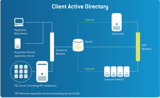
Figure 5. Overview of RayStation 10B HPC computer cluster solution.
