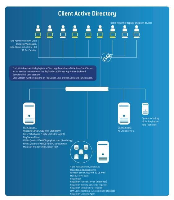
Figure 3. SQL Server. \*Note that 64 GB RAM is preferred where possible. Shared Application Server. \*\*RAM DIMM's should be installed to provide optimal RAM usage, i.e, units of 6 for Intel Xeon Scalable (192/384 GB) or units of 4 for Intel Xeon E5 (128/256 GB).
