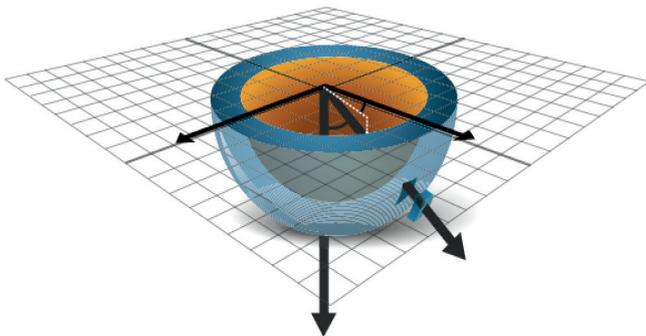
**The sphere point kernel** describes the energy distribution in a 3D spherical grid from a primary energy deposit. The figure shows a volume element in the spherical grid defined by its radius, azimuthal and polar interval. The origin of the spherical coordinate system is the interaction point. The photon enters the plot from above.
