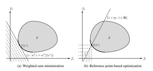
**Figure 9.** A priori multicriteria optimization methods. The dashed lines indicate level set curves for the scalarizations.
