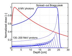
**Figure 2.** Depth-dose profiles along the central axis for a broad beam of 6 MV photons and 135–200 MeV protons. The superposition of appropriately modulated monoenergetic Bragg peaks produces a spread-out Bragg peak.
