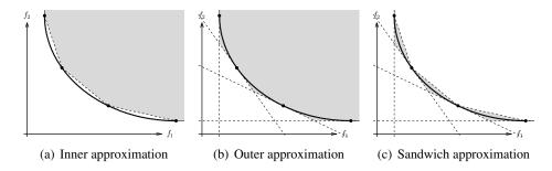
**Figure 10.** Sandwich approximation of the Pareto surface (thick solid line) using inner and outer polyhedral approximations (dashed lines).
