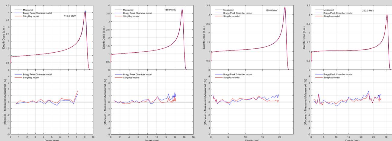
**Figure 3.** (Top panels) Measured central depth dose curves (DDCs) of  $10 \times 10$  cm<sup>2</sup> scanned single energy layers at 110, 150, 180, and 220 MeV (black curves). Corresponding calculated DDCs using RayStation 8A with beam models based on the Bragg Peak Chamber (blue) and StingRay IDDs (red) are also included. The relative difference between measured and calculated IDDs are shown below.
