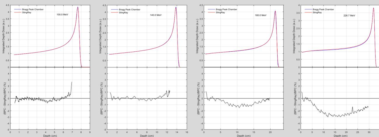
**Figure 2** (Top panels) Measured integrated depth doses (IDDs) of single spots at nominal beam energies of 100, 140, 180, and 226.7 MeV using, respectively, a Bragg Peak Chamber ( $\Phi=81.6$  mm) (blue curves) and StingRay ( $\Phi=120$  mm) detector (red). The relative difference between the IDDs of the two detectors are shown below.
